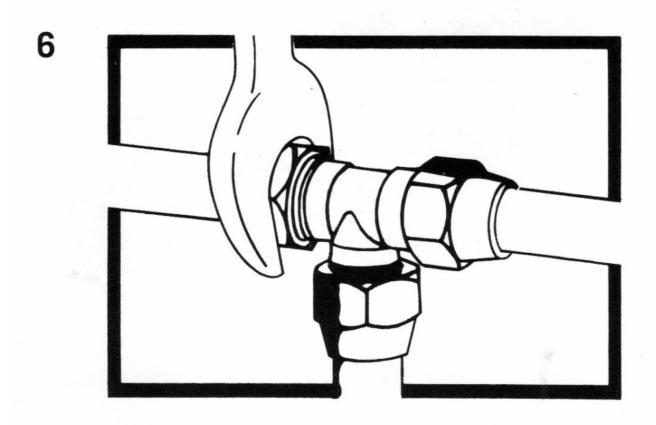
Securex joints can be assembled dry. However it is recommended that a thin film of jointing compound is applied to the external surface of the cone. This will assist in preventing
